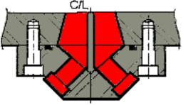
"O" ring sealed "METERGUARD" Piping Bases. MG--" Soc 45° by -- " Sec 45°
